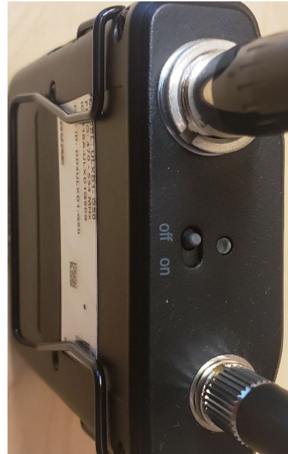
Lapel Microphone on/off switch
